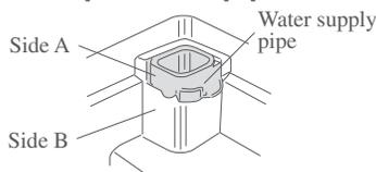
● Replace the water supply pipe. Be sure that sides A and B fit flush against each other. Otherwise, the ice maker may malfunction if the pipe is not installed properly.
