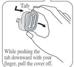
While pushing the tab downward with your finger, pull the cover off.
