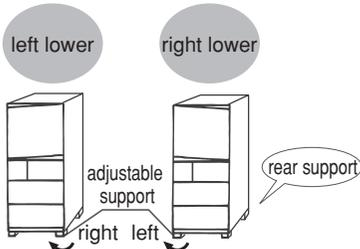
**After adjusting the supports, install the toe grille at the lowest area on the front of the refrigerator.**
