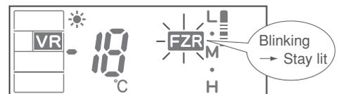
When selecting the versa compartment, the light of the temperature control display first blinks and then stays on to perform the setting. (A "beep" sound is heard).
