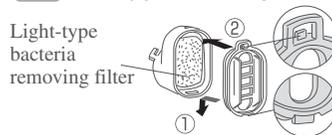
**2 Rotate the cap and catch the cap hook (1) onto the water supply pump projection (2).**
