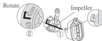
\*Make sure that the impeller is in the pump.
