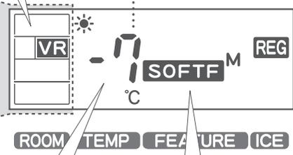
It indicates that the present temperature in the versa compartment is about -7°C.
