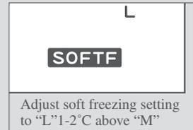
Adjust soft freezing setting to "L" 1-2°C above "M"
