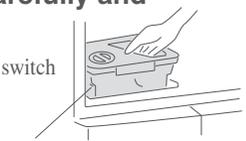
Put the water tank back to its original position.
