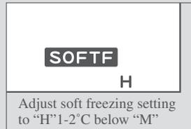
Adjust soft freezing setting to "H" 1-2°C below "M"
