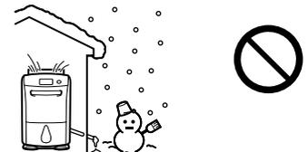
Water inside the hose may freeze and prevent the water in the tank from flowing out. The water may leak from the unit and **damage surrounding objects**.
