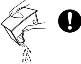
Moving the unit with water in its tank may cause the water to leak and damage the surrounding objects and in turn result in **electric shock and/or an electric leak**.
