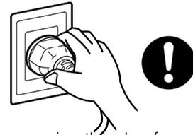
When removing the plug from the power socket, do not pull on it diagonally or by the cord as this may cause the projections/wiring to be damaged resulting in a **short circuit, electric shock or fire**.
