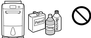
Chemicals and solvents evaporated in the air may harm the unit and cause water in the tank to leak, **resulting in damage to property**.
