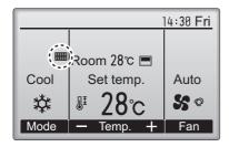
will appear on the Main display in the Full mode when it is time to clean the filters.
