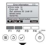
Error code, error unit, refrigerant address, unit model name, and serial number will appear.
