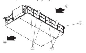
While lifting the filter knob, pull it.
