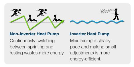
Heat pumps with old technology (fixed speed systems) used to turn on and off like an electric heater, which meant that increased amounts of power were required during this action. When your heat pump has reached the set temperature, it will ramp down but continue to circulate the room air. It is important that it does this as it aids in better heat distribution throughout your whole room; improving air circulation and enabling the system to correctly sense the whole room temperature.
