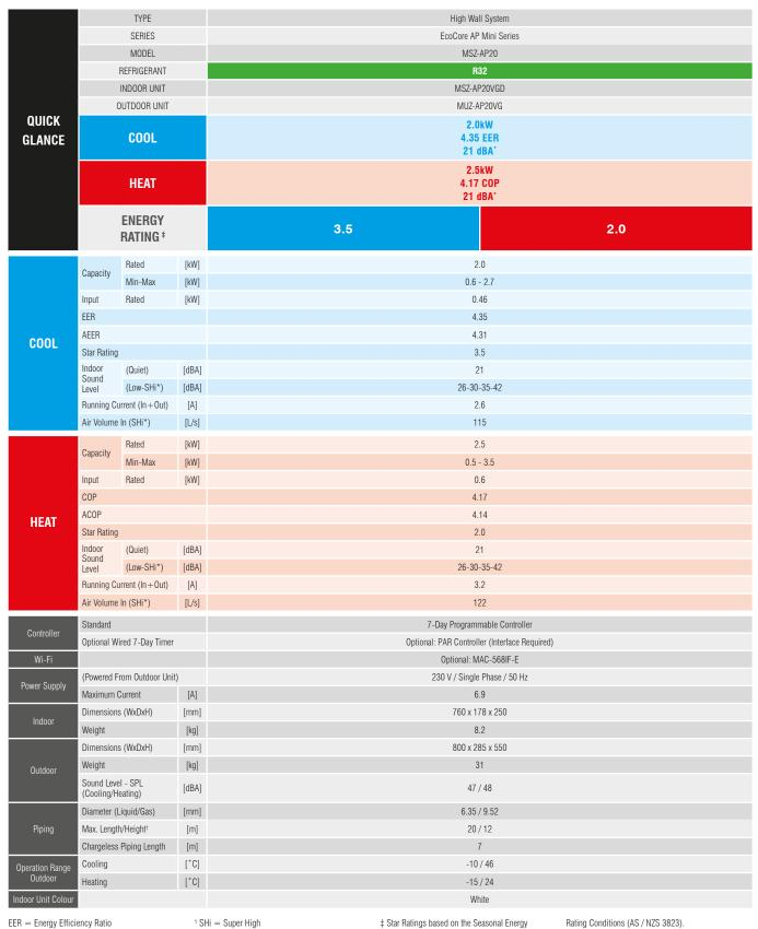
EER = Energy Efficiency Ratio COP = Coefficient of Performance AEER = Annual Energy Efficiency Ratio ACOP = Annual Coefficient of Performance SPL = Sound Pressure Level
