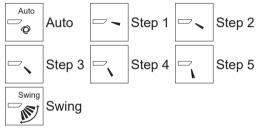
Select "Swing" to move the vanes up and down automatically.
