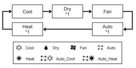
\*1 Operation modes that are not available for the connected indoor unit will not appear on the display.
