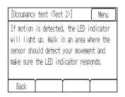
To start Test 2, touch **[Test 2]**. When movements are detected, the LED indicator will light up in blue. Walk away from the remote controller, and walk around in areas where you want the sensor to detect motions to see if it will respond correctly.
