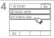
To select the brightness level of the LED indicator to be used when the brightness sensor detects "Light" or "Dark," touch the **[With Brightness sensor]** in the list.
