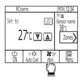
Touch the **[Fan speed]** button to go through the fan speeds in the following order. Select the desired setting.
