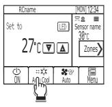
Touch the **[Operation mode]** button to go through the operation modes in the following order. Select the desired operation mode.
