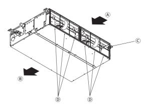
· While lifting the filter knob, pull it.
