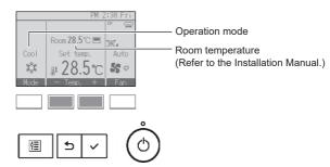
Press the [F2] button to decrease the preset temperature, and press the [F3] button to increase.
