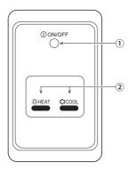
ON/OFF lamp (lit when unit is operating; unlit when unit is not operating)
