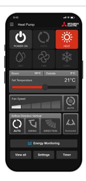
2) If your heat pump is compatible you will see [Energy Monitoring] underneath the airflow direction.
