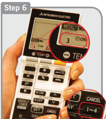
To select a 3rd and 4th time for the same day press 1-4 and ensure 3 is selected and repeat step 4. To turn OFF ensure 4 is selected and repeat step 5.
