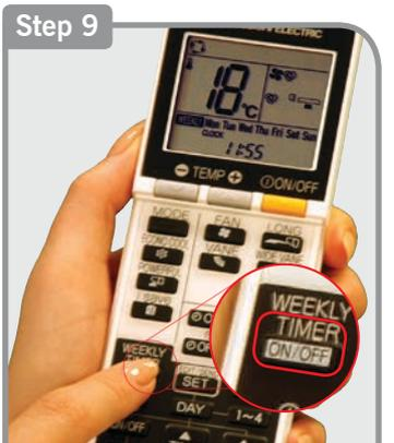
To turn your weekly timer ON (or OFF) press the WEEKLY TIMER ON/OFF button. The WEEKLY symbol will show when the timer is on.
