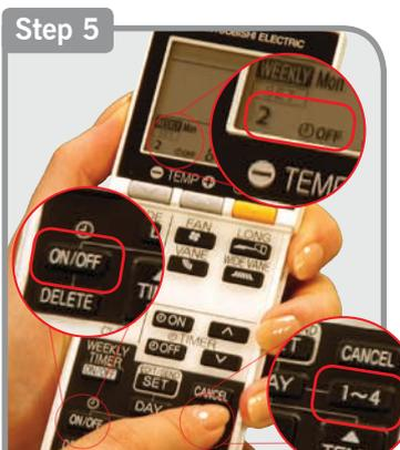
To set a time to turn your heat pump OFF on the same day, press 1 - 4, making sure 2 is selected. Select OFF, set a time to turn off by pressing TIME.
