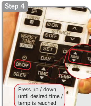
Press up / down until desired time / temp is reached
