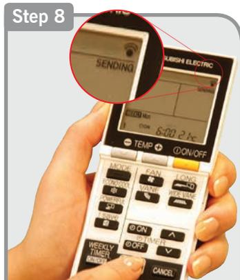
Once all ON/OFF Temp requirements have been set select the Edit/Send Button. Point the remote at the heat pump until the "sending" logo disappears.
