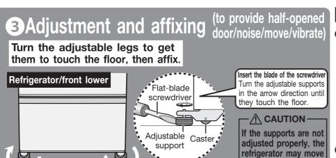
\* Before adjusting, please pull the leg cover to the front and remove it.
