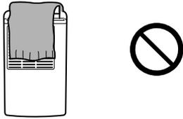
This results in poor ventilation and may cause **heat generation/fire**.
