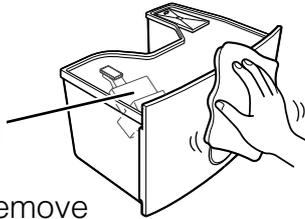
The unit draws in dust present in the air, and this may cause the tank **to gradually become dirty**. If the dirt does not come off easily, wash with cold or warm water, then wipe with a soft, dry cloth.
