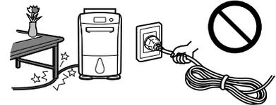
The cord may be damaged resulting in **fire or electric shock**. (Keep pets from biting the cord.)
