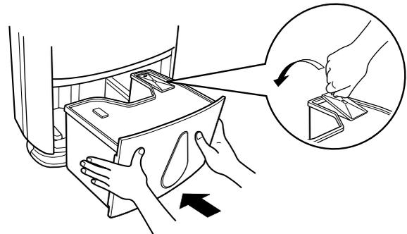
Check that the lid and guard are secure. Slide the tank in with both hands (you should hear a beep).
