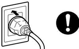
If the plug is not fully inserted into the socket, dust may gather on the connectors which may cause **fire and/or electric shock**.
