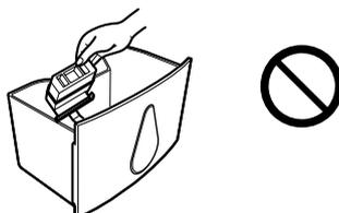
The floating element will not be able to detect a full tank resulting in water leakage, which may **damage surrounding objects or cause electric shock and/or an electric leak**.
