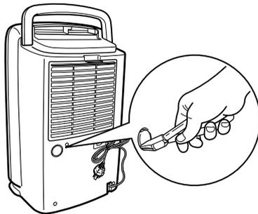
Use pincers to cut away the three securing ribs of the continuous drainage outlet. Remove carefully without letting any debris fall inside.
