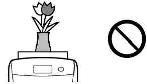
Water may leak into the unit adversely affecting electric insulation and cause **electric shock and/or fire by short-circuiting**.
