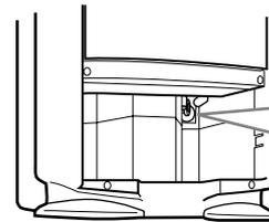
Confirm that the hose is securely attached and does not leak.
