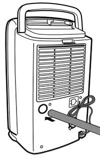
Feed the commercially available hose (ID 15 mm) into the drainage outlet while keeping the stopper pressed
