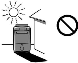
This may cause **overheating, electric shock and/or fire caused by an electric leak**.
