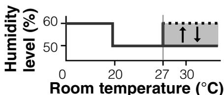
The unit automatically controls airflow to counter excessive room temperature/humidity. It activates the blower at high temperatures.
