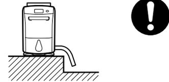
The water in the tank may leak and damage **surrounding objects**.
