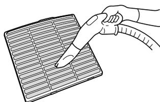
Run a vacuum cleaner lightly over the air filter surface to remove the dirt.
