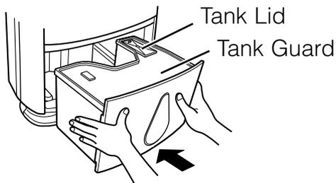
Check that the lid and guard are secure. Slide the tank in with both hands.
