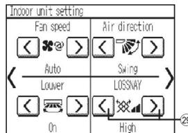
\* Indoor unit fan may operate even when the LOSSNAY unit is operated individually, depending on the models of the indoor unit and the LOSSNAY unit.
