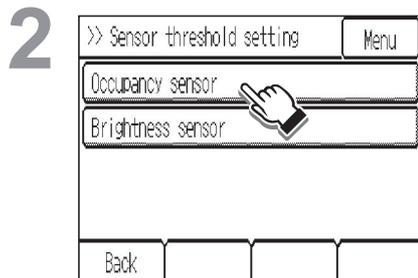
To set the detection sensitivity level of the occupancy sensor, touch **[Occupancy sensor]** in the list.
