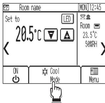
Touch the **[Operation mode]** button to go through the operation modes in the following order. Select the desired operation mode.
