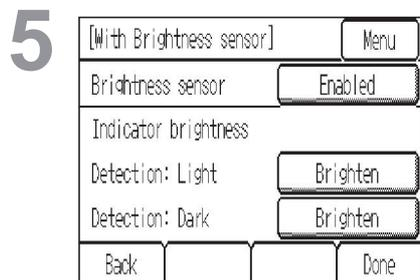
To use the brightness sensor for switching the brightness of the LED indicator, touch the **[Disabled]** button to change it to **[Enabled]**.
