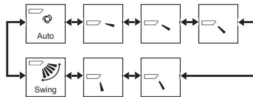
Select "Swing" to automatically swing the airflow direction.
