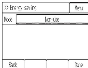
Touch the **[Mode]** button to select one of the following energy-save control modes that reduces energy-consumption during vacancy. The default setting is “Non-use.”
